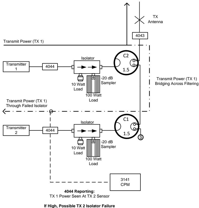
Figure 5 – Isolator Characterization through Adjacent Transmitter 4044 Sensor Data
