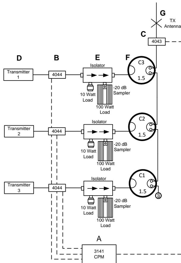
Figure 1 - CPM Integrated in T-Pass Combiner System
