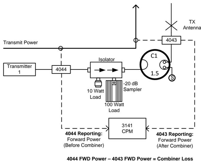
Figure 4 – Combiner Characterization through Forward Power Comparison
