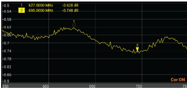
Figure 11 Interpreting Cable Loss Measurement
