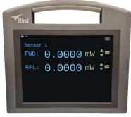
One Sensor Operation — The 4421A RF Power Meter will display the RF power measurements of one RF Power Sensor. The sensor may be connected to either of the Sensor connectors, see <a href="#">"4421A Controls and Indicators"</a> on page 6.
