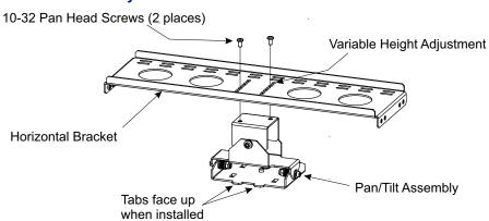
2. Position the Horizontal Bracket over the Pan/Tilt Assembly.
