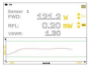
Sensor Measurement with Graph Displayed
