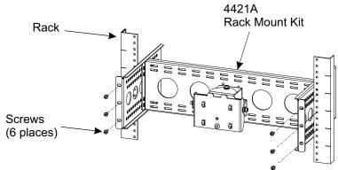
The Rack Hardware Kit provides various screws and nuts for the four most common types of racks.
