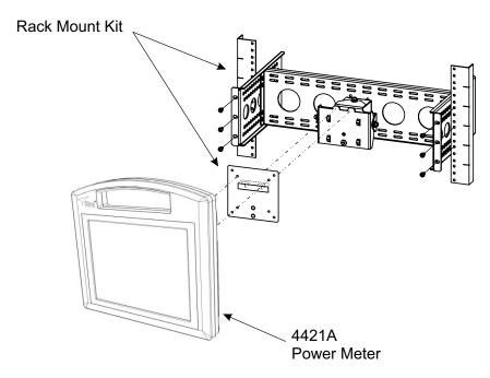
After the Rack Mounting kit is installed in a rack, the 4421A can be removed and reinstalled without the use of any tools.
