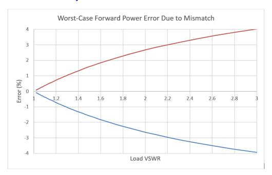
Figure 13 Sensor Accuracy Vs. Load VSWR
