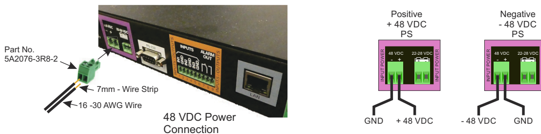
Figure 9 48 VDC Wiring Diagram
