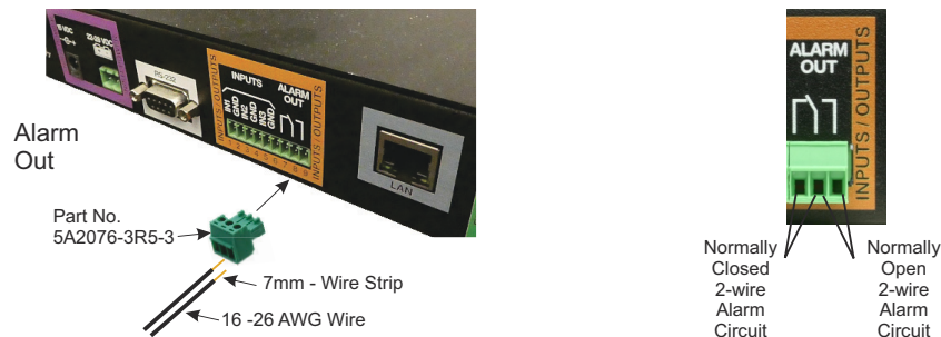
Figure 6 Alarm Out Connector Installation
