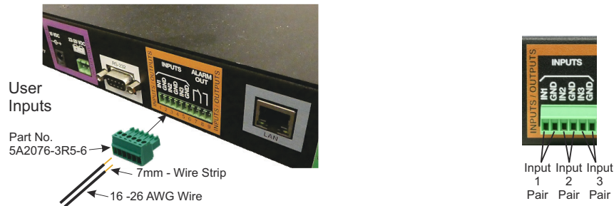
Figure 7 User Input Connector Installation
