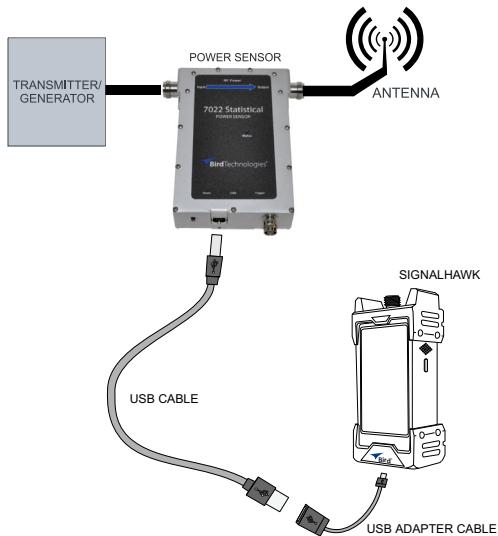
Figure 18 Power Sensor Connections
