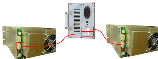
Backup Power for Two Master Units
