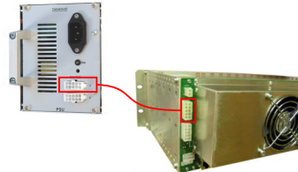
Primary Power for One Master Unit
