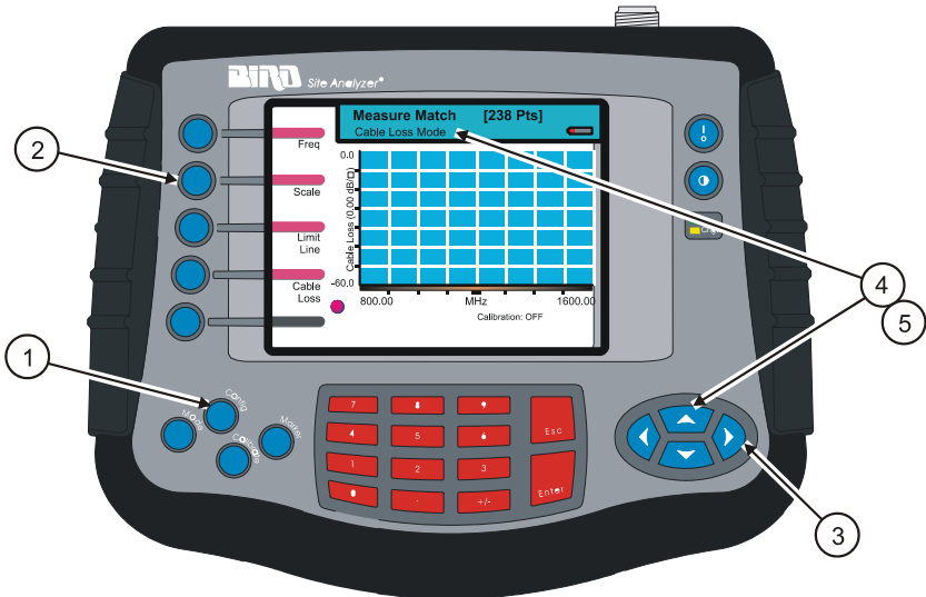
Figure 18 Set Up for Cable Loss Measurement
