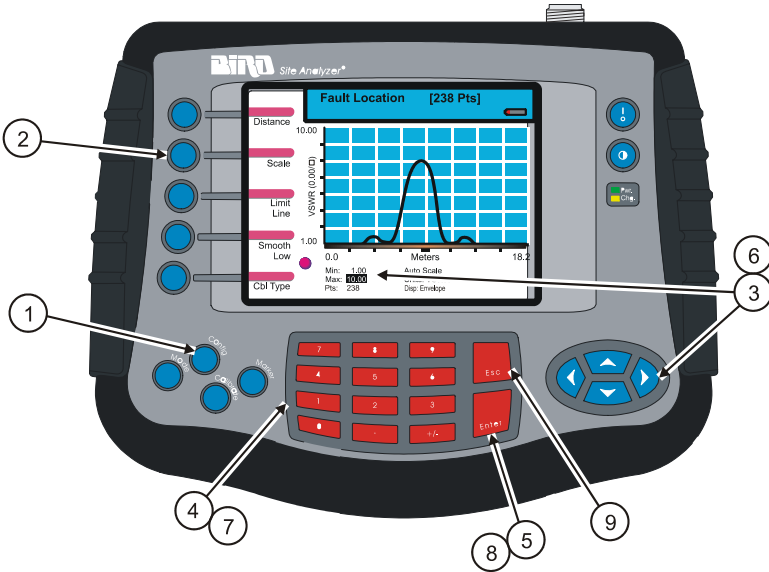
Figure 28 Setting Fault Location Scale Limits Manually
