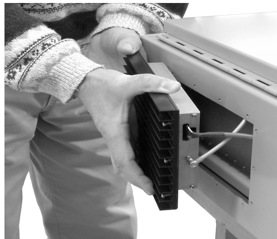
Figure 13: Slide amplifier towards top of cabinet to remove lower cables.
