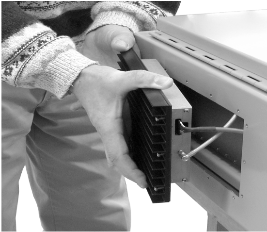
Figure 12: Slide amplifier towards top of cabinet to remove lower cables.
