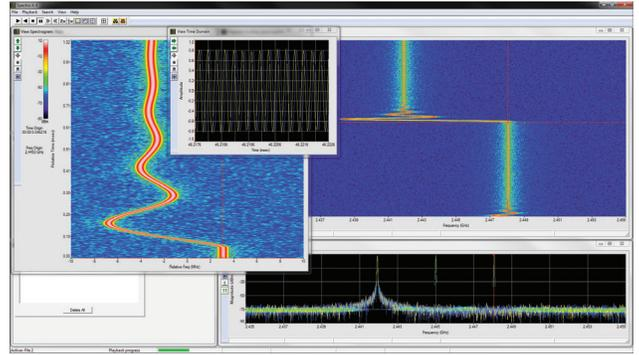
Spectrogram time windows positioned in time and frequency by marker placement.
