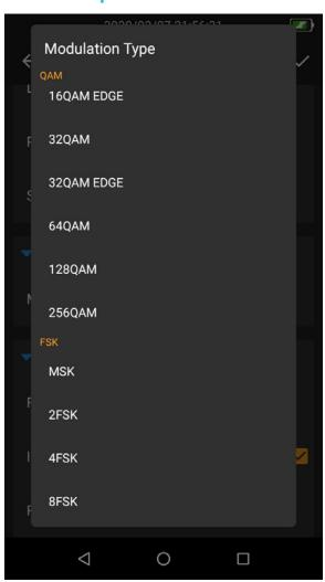
**The Custom Digital Modulation** module gives you the ability to generate a wide variety of digital signals that can be used to test devices' ability to process digitally modulated signals.
