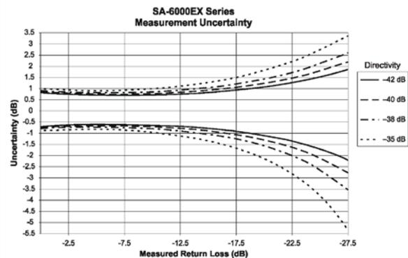
Due to the impact of directivity and the way VSWR and return loss are calculated, there is no easy specification for error on either of those measurements that can be used for every application. The specific accuracy is dependent upon the performance of the system being measured.
