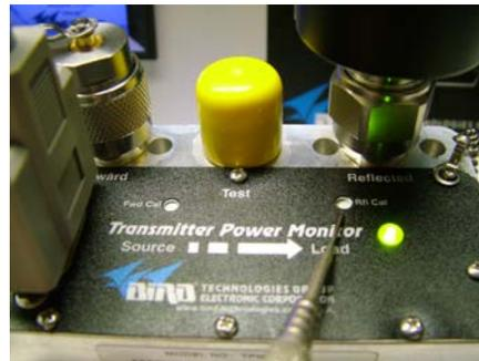
Using either a voltmeter or a 3140A8 meter, measure the power coming from the DB9 connector on the TPM. When using the 3140A8, simply confirm that the power is on and read the power on the forward meter. When using the voltmeter, you will need to set up the system using the 9 pin diagram below. Make sure that Vcc is supplied so that the TPM power light is on.
