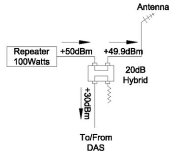
Figure 2c. Hybrid Coupled Repeater
