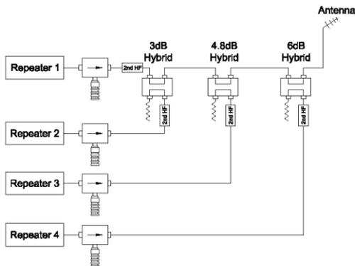
Figure 3. 4-Channel Progressive Hybrid Combiner
