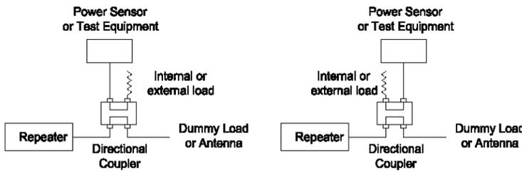
Figure 2a. Hybrid Sampler configured to measure Incident power
